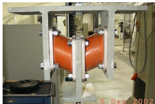
SDI-R test at the University Munich
