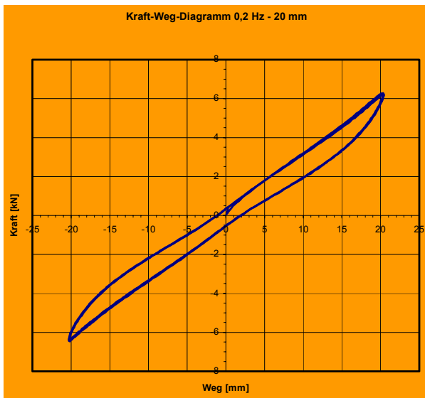
SDE-R test with hysteretic loop
